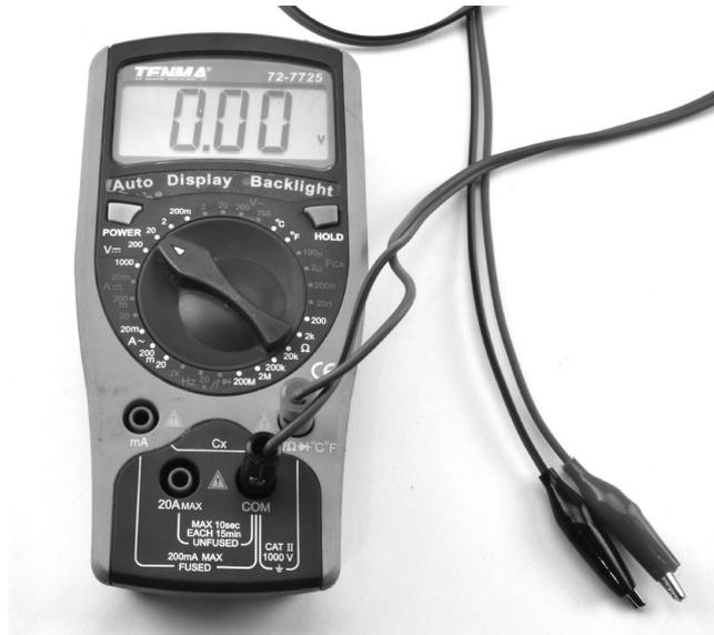
3-10 A low-cost digital multimeter.
